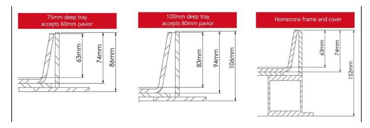
Homezone covers are used for 'shared surface' areas, where the demarcation between pedestrians and drivers is minimised. These areas use deep paving materials rather than typical road construction materials possess low speed limits. Because of this, they qualify as B125 areas because they feature slow moving traffic.
